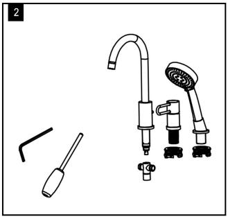
2. As shown in the picture, first remove the three sets of fixing parts, and then follow the removal steps to pass through the fixing sets from the bottom and connect them to the main body.
