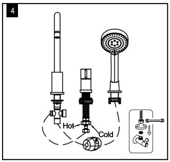
4. As shown in the figure, connect the water inlet hose to the hot and cold water valve, and finally install the gravity ball on the pull-out shower pipe.
