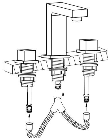
Connect the pipe of spout and two handles
