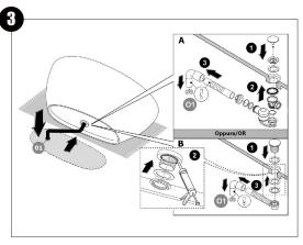
3.Install the water pipe according to the schematic diagram, and then confirm whether the water pipe is connected properly and will not leak. Finally, insert the water pipe into the floor drain
