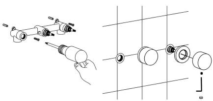
4. Install outlet pipe (Convovle Teflon tape round screw).
