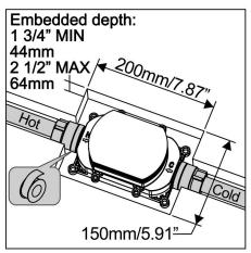
1. Connect the embedded box with the water inlet pipe, and connect the hot water pipe with the word "H" on the box body, and connect the cold water pipe with the word "C"
