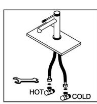
5. Attach flexible hose to water supply.
