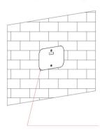
Tile surface and plastic box surface flush transparent protective cover protruding from the tile surface
