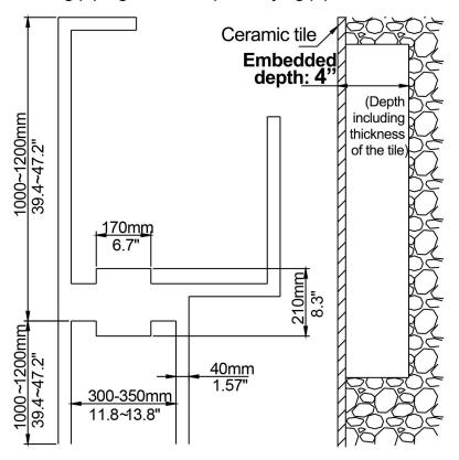
2. Install the main body, water inlet and outlet pipes.
