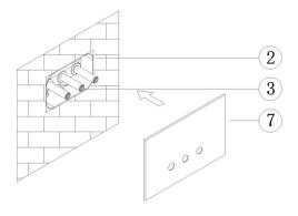
2. Fix the pre-buried main body with reference to the level to ensure the level, the water pipe is connected to the water for 24 hours to ensure sealing; do not remove the transparent protection cover when sealing the wall with cement to avoid splashing cement to the copper parts threads.
