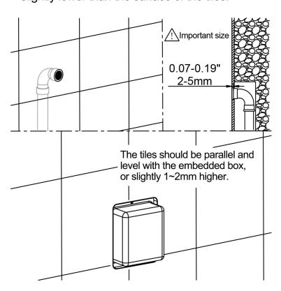
4. Stick the tiles, remove the protecting cover,install the cover plate and diverter.
