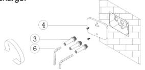
6. Insert the main body of the shower head according to the corresponding inlet parts and lock the hexagonal screws with a hexagonal key, and the installation is complete.
