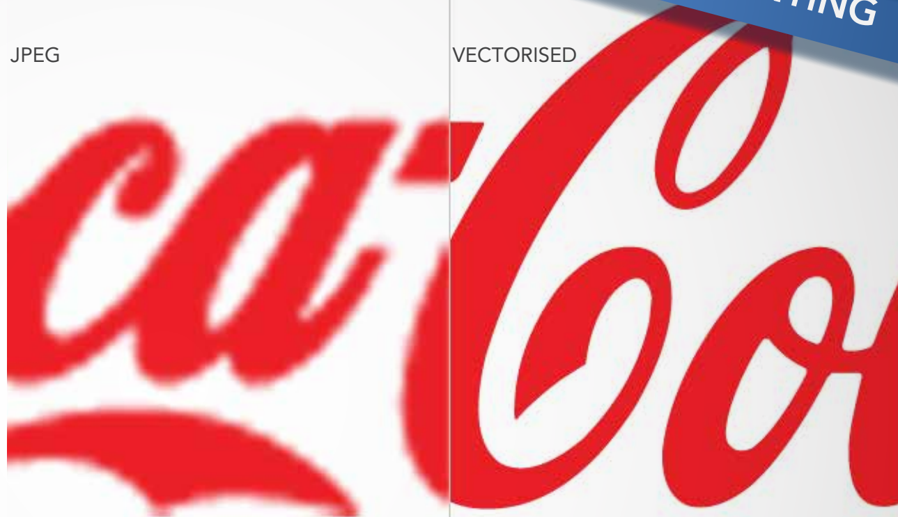
Above left is a JPEG, showing poor quality of a low resolution image. The above right is a Vectorised image making it perfect for reproduction.
