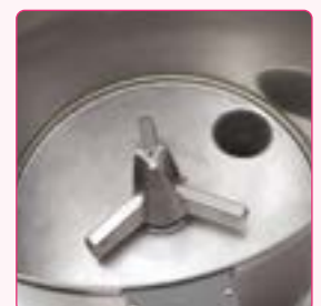
Residual water drain
