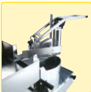
Lever operated hopper
