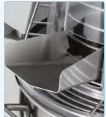
Removable spout to add ingredient during process
