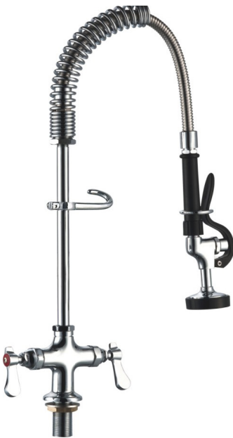
MODEL GXR-MN13B Pre-rinse Faucet - Deck Mount Deck mount with 7" riser and 22" flexible stainless steel hose GXR-90S spray valve *WRAS approved
