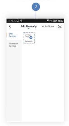
Select your WiFi network and set the password (5GHZ Wi-Fi is not compatible with the Delta-WIFI Module)
