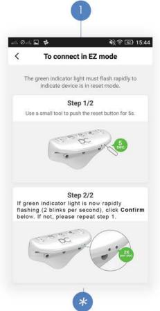
The indicator should start rapidly flashing.
