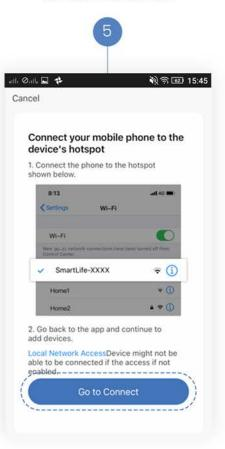
On the Wi-Fi selection screen, look for the SmartLife-XXXX device hot spot and select it. Once the device is added successfully.
