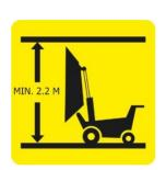
The machine may only be transported using a vehicle with sufficient headroom as there is a risk of serious injury and damage to the operator,
