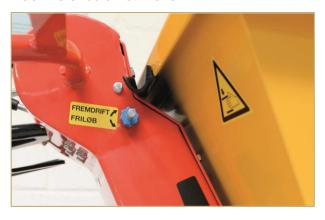
Check that the valve button is not damaged.
