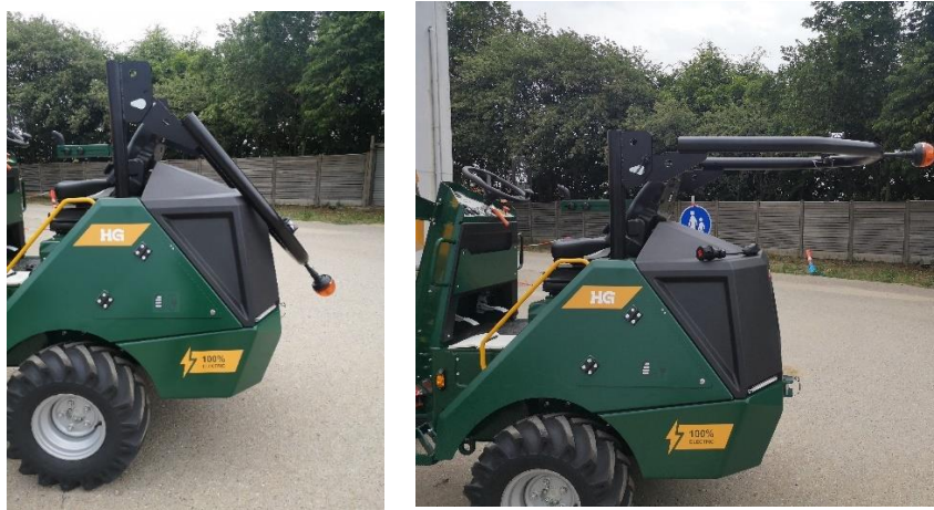
Figure 12: Crash bar lowered
