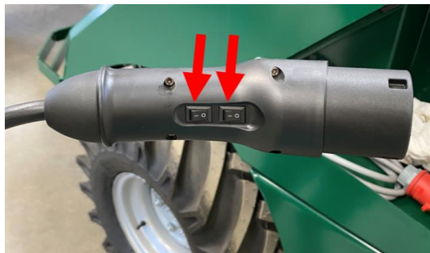
Figure 57: Switches on charger
