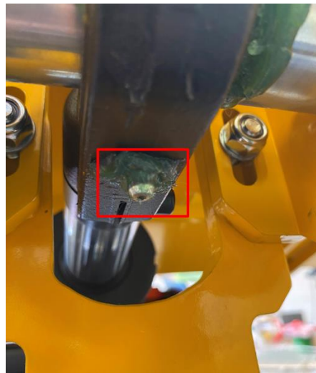
Figure 75: Grease nipple under container by rotation lock
