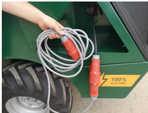
Figure 54: Charging cable with extension
