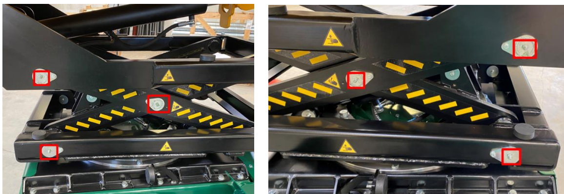
Figure 77: Grease the nipples on the right and left side of the swivel arms
