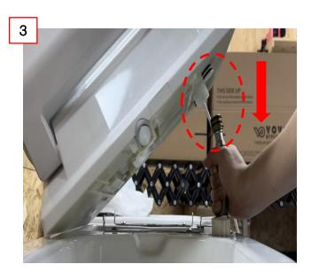
③ Pull the hose down to completely disconnect it.
