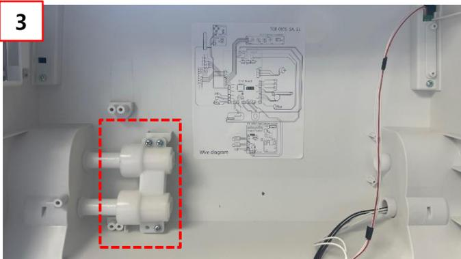
③ Screw the 3 screws to fix the DAMPER
