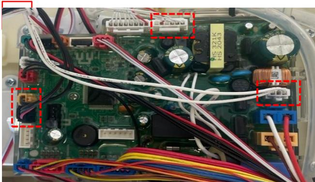
① Detach the SEAT harness that is connected to PCB
