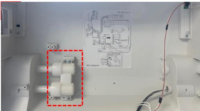
③ Unscrew the 3 screws from the DAMPER inside the COVER BASE
