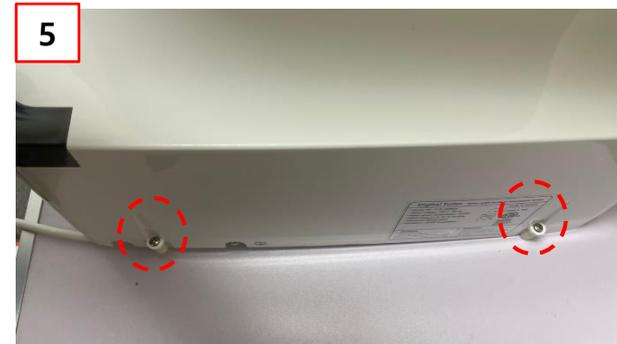
⑤ Screw the 2 screws back using a Phillips head driver.
