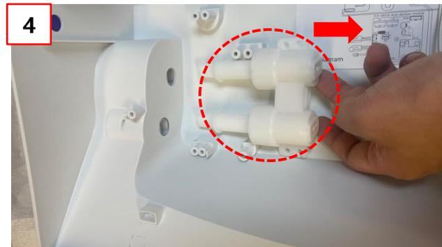
④ Detach the DAMPER in the direction shown in the photo.
