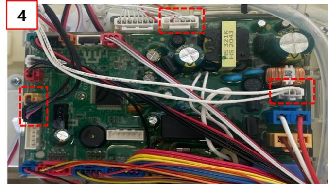
④ Reattach the harness from MAIN PCB and SEAT.
