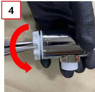
④ Detach the strainer filter (white part) from the strainer by rotating it clockwise
