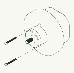
Tuck wires into J-Box and attach Sconce Assembly **(D)** to Universal Crossbar **(F)** with Taku Screws **(C)**.
