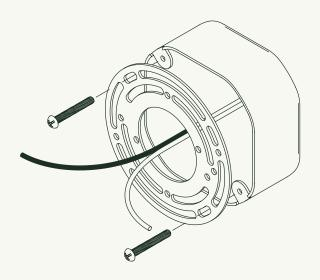
Attach Universal Crossbar **(F)** to J-Box using J-Box Screws **(E)**. If a Ground Wire is present in the J-Box, attach it to the Universal Crossbar **(F)** using the green Ground Screw.
