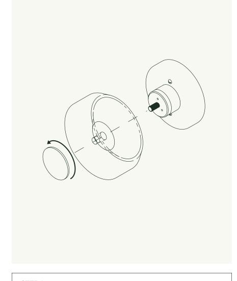
Unscrew Cap (A) and slide Glass Shade (B) off of Sconce Assembly (D).
