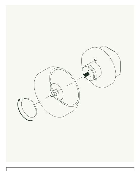
Slide Glass Shade (B) onto Sconce Assembly (D) and fasten with Cap (A).
