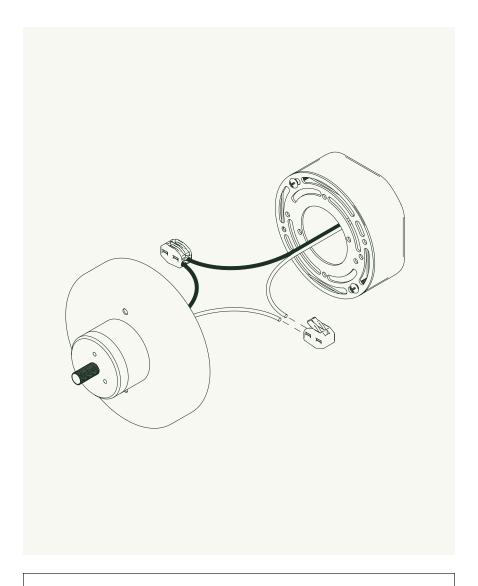
Using Lever Nuts (G), connect Sconce Assembly (D) to 120VAC power.
