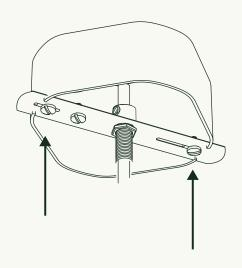
Fasten Crossbar Assembly (B) to J-Box with J-Box Screws (C).
