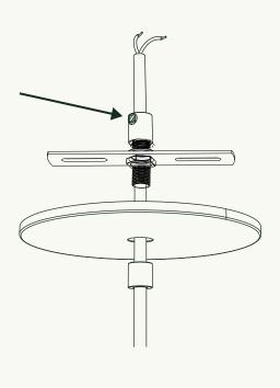
Thread pendant cord through Bushing **(E)**, Canopy **(D)**, and Crossbar Assembly **(B)** in that order. Be careful not to snag the cord on these items – the cord will fray. Loosen strain relief set screw at the top of the Crossbar Assembly to allow the cord to pass by.
