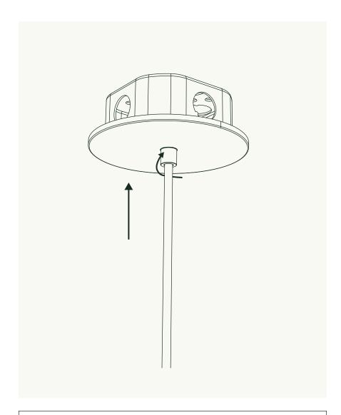
Carefully slide Canopy **(D)** and Bushing **(E)** up to Crossbar Assembly **(B)** without snagging cord. Thread Bushing onto the Crossbar Assembly to secure the Canopy snug against the mounting surface.
