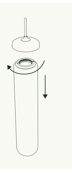
Unthread the glass shade from the socket assembly while holding the socket assembly stationary. Do not allow the cord to twist.
