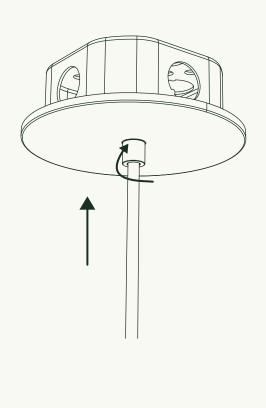
Carefully slide Canopy **(D)** and Bushing **(E)** up to Crossbar Assembly **(B)** without snagging cord. Thread Bushing onto the Crossbar Assembly to secure the Canopy snug against the mounting surface.
