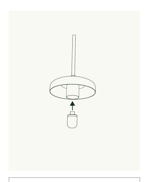
Install the Light Bulb **(G)** by pushing it into the socket until seated. Polarity of the pins does not matter.
