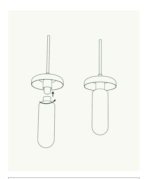
Thread Diffuser **(H)** onto threaded socket until its shoulder just touches the socket cup, then stop. Do not tighten Diffuser.
