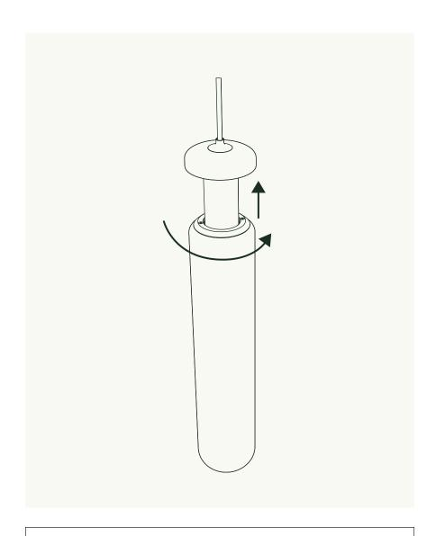
Re-install the glass shade by threading it onto the socket assembly until seated. STOP THREADING ONCE THE SHADE IS SEATED. OVERTIGHTENING THE SHADE WILL CAUSE THREADS TO SEIZE AND LOCK UP.
