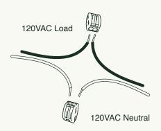
Using Lever Nuts **(A)**, connect pendant wires to 120VAC power. If a Ground Wire is present in the J-Box, attach it to the Crossbar using the green Ground Screw.
