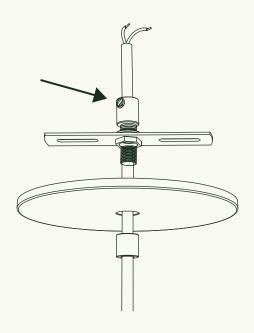
Thread pendant cord through Bushing (E), Canopy (D), and Crossbar Assembly (B) in that order. Be careful not to snag the cord on these items – the cord will fray. Loosen strain relief set screw at the top of the Crossbar Assembly to allow the cord to pass by.
