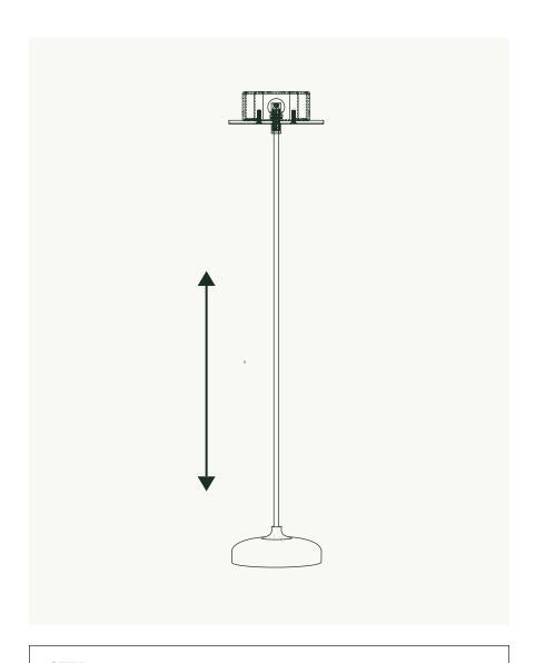
Set desired cord height by tightening the strain relief set screw at the top of the Crossbar Assembly **(B)** back down against the cord.
