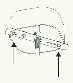
Fasten Crossbar Assembly (B) to J-Box with J-Box Screws (C).
