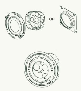
Install in Mud Ring with 2-¾" hole spacing or use the provided Universal Crossbar (**D**). If using a Universal Crossbar, fasten to the J-Box with J-Box Screws (**B**). Orient the Universal Crossbar so that its threaded holes with 2-¾" spacing are horizontal.
