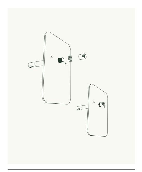
Assemble the sconce mount. Pull the Pipe Assembly **(H)** through the Backplate **(F)**. Thread the Hex Nut **(E)** and Strain Relief **(C)** onto the nipple.
