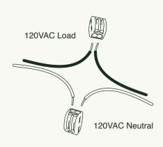
Using Lever Nuts **(A)**, connect pendant wires to 120VAC power. This fixture does not require a ground connection.
