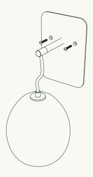
Fasten the sconce assembly to the Universal Crossbar or Mud Ring using the provided Slotted Screws **(G)**, tucking any excess cord into the J-Box.
