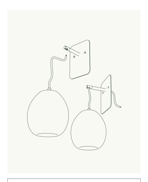
Pull the cord through the sconce assembly. Set it to desired height and tighten the set screw on the Strain Relief **(C)**.
