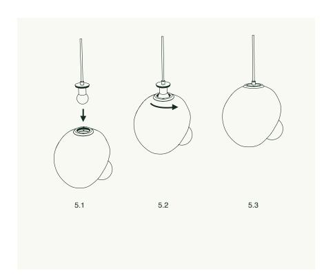
5. Re-install the glass shade by threading it onto the socket assembly until seated. STOP THREADING ONCE THE SHADE IS SEATED. OVERTIGHTENING THE SHADE WILL CAUSE THREADS TO SEIZE AND LOCK UP.
