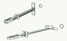
Slide Zip-Toggle **(A)** finger grips in opposite directions to flatten out the metallic part. Then slide it into the hole in the wall until the metallic part is all the way through the drywall and inside the hollow wall.
