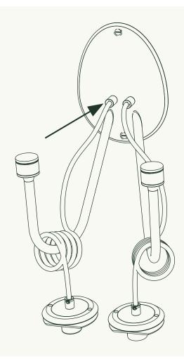
Locate an Ontologia Light **(F)** and pass its cord through one bushing on the face of the Sconce Body **(D)**. You may need to loosen the set screw on the backside of the Sconce Body to get the cord to pass through. Be careful not to fray the cord. When desired cord length is achieved, tighten down the set screw against the cord. Repeat for the other Ontologia Light.
