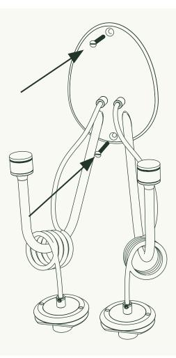
Place Sconce Body **(D)** over the J-Box and zip-toggles, tucking all wires into the J-box. Thread Mounting Screws **(E)** into the zip-toggles and tighten to secure the Sconce Body to the wall.
