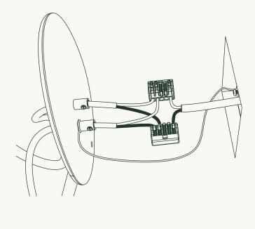
Using 5-way Lever Nuts **(B)** connect Ontologia Lights **(F)** to 120VAC power. Connect the green ground wire to the J-Box ground wire with a 2-way Lever Nut **(C)**. Cut and strip wire as required so it will fit in the J-Box.
