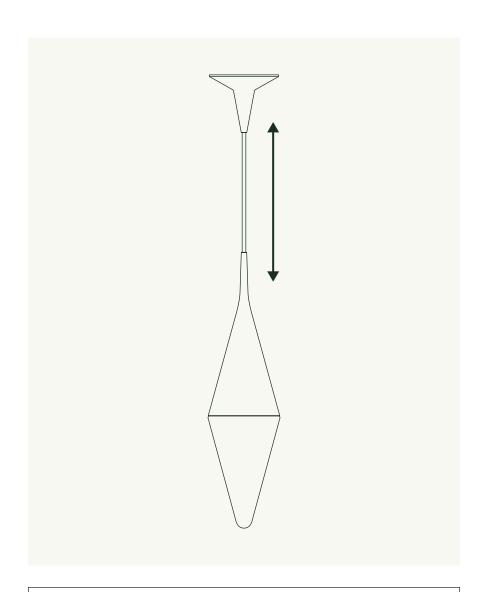
Set desired cord length by adjusting Strain Relief (B). Loosely coil extra cord inside J-Box.
