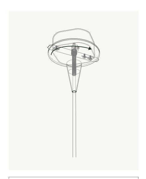
Carefully slide Canopy **(E)** up to Crossbar Assembly **(C)** without snagging cord. Thread Canopy **(E)** onto Cross-Bar Assembly **(C)** until snug against ceiling.
