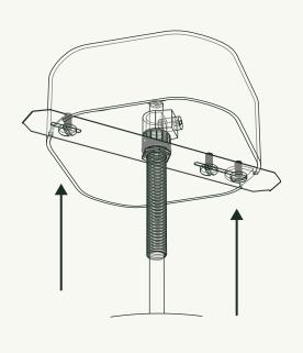
Fasten Crossbar Assembly (C) to J-Box with J-Box Screws (D).
