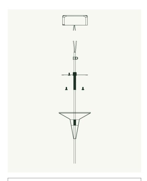
Thread pendant cord through Canopy (E), Crossbar Assembly (C) and Strain Relief (B) in that order. Be careful not to snag the cord on these items—the cord will fray. Tighten Strain Relief (B) against cord using set screw.
