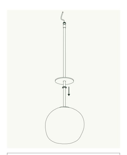
Unscrew the knurled ring from the Hang-Straight **(E)** and carry it down the Pipe **(F)** to rest on the Lacuna Pendant **(G)**. Slide the Canopy **(D)** onto the Pipe and pass it down as well. Be careful not to scratch the finish.
