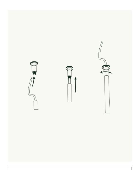
Pass the pendant cord through the Hang-Straight **(E)** and screw the Hang-Straight onto the Pipe **(F)**.
