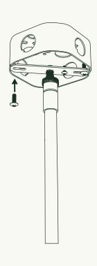
Fasten the Crossbar Assembly **(B)** to the J-Box with J-Box Screws **(C)**.
