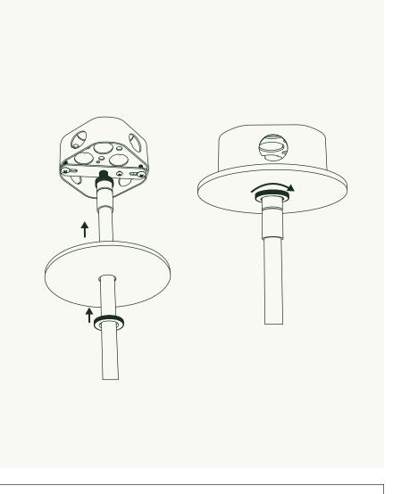
Carefully carry the Canopy **(D)** and Knurled Ring back up to the Hang-Straight **(E)**. Thread the Knurled Ring onto the Hang-Straight, securing the Canopy snug against the mounting surface.
