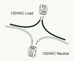
Using Lever Nuts (A), connect pendant wires to 120VAC power. If a Ground Wire is present in the J-Box, attach it to the Crossbar (B) using the green Ground Screw.
