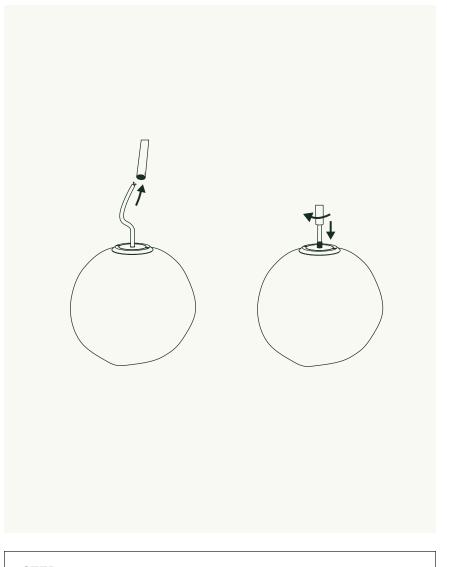
Pass pendant cord through the Pipe **(F)** and screw the Pipe onto the threaded rod on the top of the Lacuna Pendant **(G)**.
