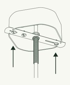
Fasten Crossbar Assembly (C) to J-Box with J-Box Screws (D).
