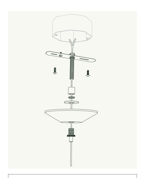
Thread pendant cable through Canopy **(H)**, Washer **(G)**, ¼ IPS Hex Nut **(F)**, Coupling **(E)**, and Crossbar Assembly **(C)** in that order.
