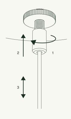
Adjust cable length as desired with Cable Gripper (I).
