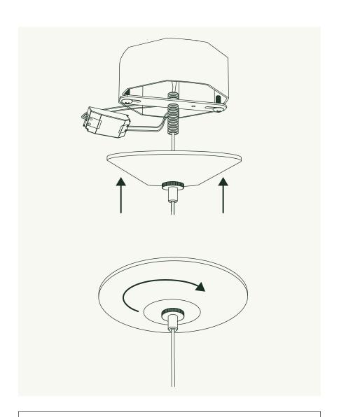
Carefully slide Canopy **(H)** up to Crossbar Assembly **(C)**. Tuck wired LED Driver **(B)** into Canopy and thread Canopy until snug against ceiling.
