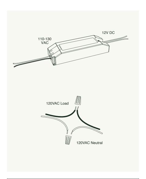
Connect junction box hot wire (black) to the VAC Line input of the driver with a Lever Nut **(A)**. Connect junction box neutral wire (white) to the VAC Neutral input of the driver with a Lever Nut.
