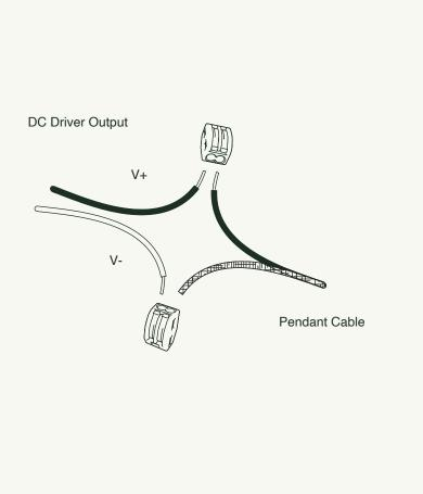
Connect black wire of pendant cable to the V+ DC output of the driver using a Lever Nut (A). Connect metal braid of pendant cable to the V- DC output of the driver using a Lever Nut.
