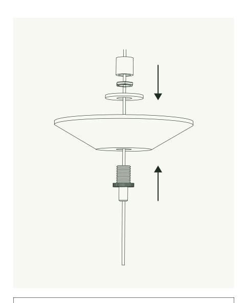
Seat Canopy **(H)** and Washer **(G)** onto the Cable Gripper **(I)**, then thread ¼ IPS Hex Nut **(F)** onto Cable Gripper. Tighten against Canopy. Thread Coupling **(E)** onto Cable Gripper.
