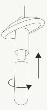
Thread Frosted Diffuser (C) onto socket of Armature Assembly (B). We recommend leaving 1-34" to 2" of Frosted Diffuser exposed beyond the socket cup.
