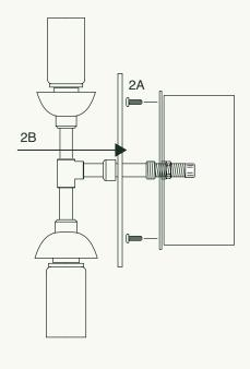
**2A.** Screw Crossbar **(H)** to junction box with J-Box screws **(F)**. Use fingers and a screwdriver held at an angle.
