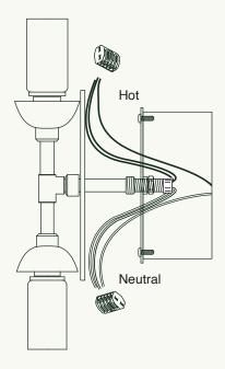
Pull wires through wall opening and wire black to hot and white to neutral using the provided Lever Nuts (E). If a ground wire is present in the junction box, attach it to the Crossbar (H) using the green ground screw. Tuck wires into junction box and repeat steps from 2B to secure fixture to the wall.
