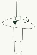
Unthread bushing above wood cover on Armature Assembly (B).
