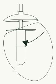
Pull bushing and wood cap away from metal hanger. Slide Glass Shade **(A)** over hanger.
