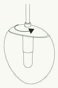
Tighten bushing against wood cover, securing Glass Shade (A).
