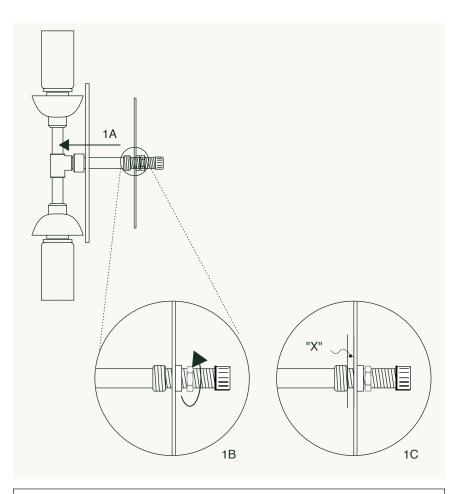
1A. Unthread bushing from its resting place on the Armature Assembly (B) pipe and slide it up the pipe. Then slide the backplate up the pipe as well.
