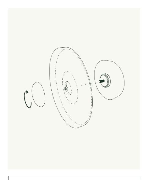
Slide on Glass Shade **(B)** and twist Wood Cover **(A)** onto pipe until finger tight.
