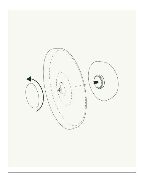
Unscrew Wood Cover (A) and slide Glass Shade (B) off of pipe.
