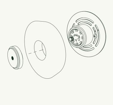
Slide LED Lens (D) and Wood Ring (C) off of LED Module (F).
