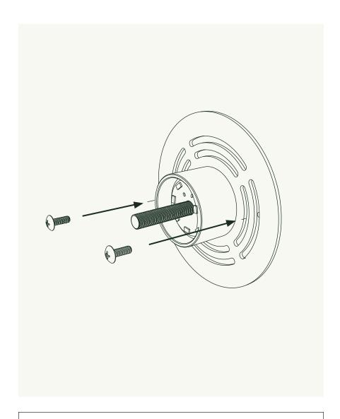
Attach LED Module **(F)** to standard 4" J-Box with two J-Box Screws **(E)** through the universal crossbar.
