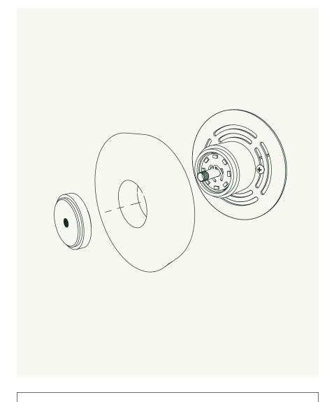
Slide Wood Ring **(C)** onto LED Module **(F)**. Slide LED Lens **(D)** onto LED Module **(F)** until Wood Ring is secured to the wall.
