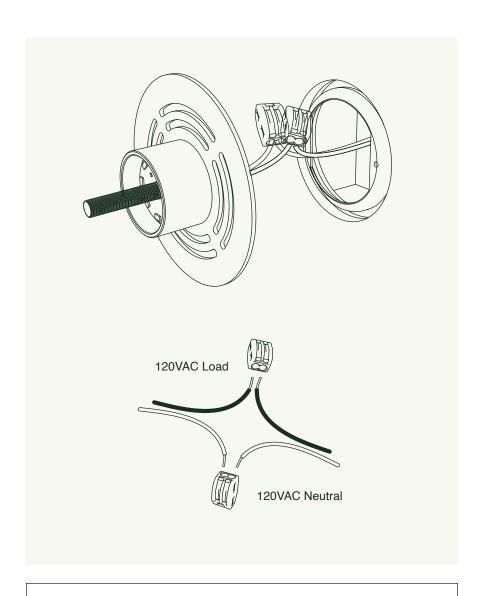
Using Lever Nuts (G), connect LED Module (F) to 120VAC power.
