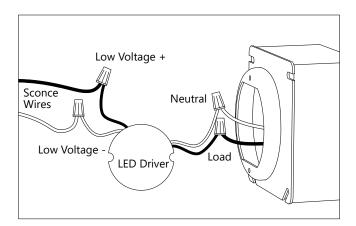
2. Wire LED driver to 120VAC power and then to the Sconce according to the diagram on the left.
