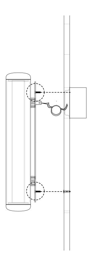
4. Using your fingers first to fit screws and then the provided stubby hex key, alternate tightening the two screws, threading each screw 3/4 turn at a time. Continue until sconce is tight against the wall.
