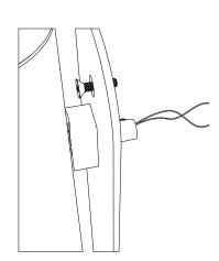
3. Thread hex screws through the backplate. Align these screws with the top mud ring hole and drywall anchor Carefully tuck wired LED driver into JBox.
