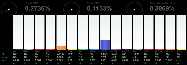
Analysis Method: SOP.T.30.031.TN & SOP.T.40.031.TN Expanded Measurement of Uncertainty: Flower Matrix d9-THC: ± 0.100, THCa: ± 0.124, TOTAL THC ± 0.112. These uncertainties represent an expanded uncertainty expressed at approximately the 95% con dence level using a coverage factor k=2 for a normal distribution.
