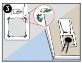
Optional: Use **Smash Plate** as guide. Secure to ceiling using pins as a stamp.
