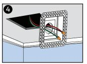
Disconnect power and feed wires through ceiling and **Mount**.
