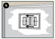
Insert **Body** and slide into place until secured.
