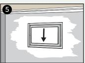
Insert **Tray** by sliding perpendicular to **Body**
