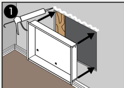
Apply adhesive around drywall opening and fit the **Body** inside.
