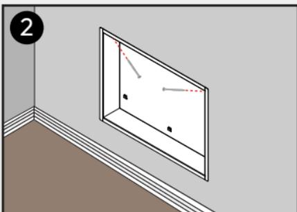
Ensure flange is flat to the wall. Use screws to fasten to studs.
