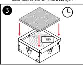
Apply silicone in **Tray**. Set pre-cut **Tray** insert into place. Allow time to cure.
