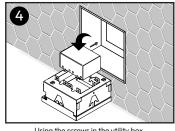
Using the screws in the utility box, fasten the utility box to the rear of **Body** component.
