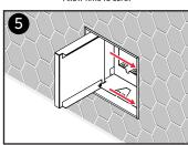
Re-engage **Body** by aligning latches and pushing firmly towards the inner corners opposite of the hinged **Door**.
