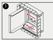
Disengage **Body** from **Base** by pushing firmly towards the hinged walls' innermost corner with the **Door** ajar.
