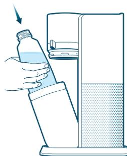
**3** Insert the Glass Carbonating Carafe / Plastic Carbonating Bottle into the carbonating flask
