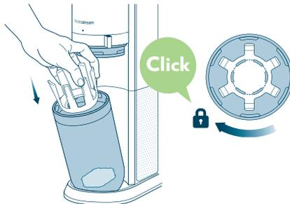
**4** Return plastic bottle holder and twist clockwise to lock into place
