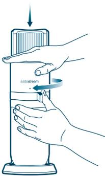
**6** Turn the lever to the left until it reaches the locked position mark
