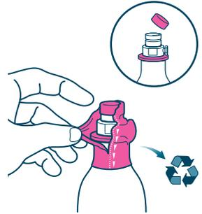
**1** Remove the seal and pull off the cap
