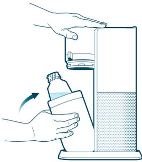
**4** Return the carbonating flask to the upright position
