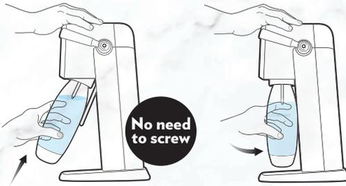
**3** Insert bottle neck into the Snap-Lock system. Push it **up** and then **back**.
