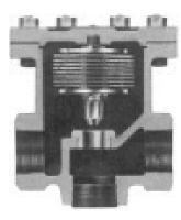
Figure 1. B SeriesThermostatic Steam Traps
