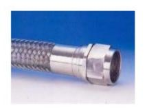
High pressure smooth bore PTFE hose (5000 PSI) is used in a variety of applications, such as hydraulics, compressed gases, R.I.M. (reaction injection molding machines), urethane transfer and hot melt glue. Series HP hose has a conductive PTFE core with a single layer of stainless steel wire braid in the smaller diameters. Larger diameters are double-braided.
