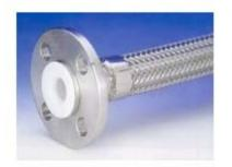
This rugged hose has a smooth liner that provides high flow rates and is easily cleaned. The metal hose provides a long flexing life and is very durable. The inner line of PTFE is locked in place and then flared over the flange faces. Series MTL hose applications include acid transfer, chemical transfer and elimination of vibration in piping systems.
