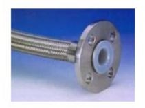
Flared tube hose is used in applications where internal corrosion of the fittings or metallic contamination of the transfer chemical is a concern. FT series flared tube hose is a convoluted PTFE hose available in non-conductive or conductive PTFE. The PTFE tubing is flared over the face of the flange, isolating the flange from the transfer chemical.
