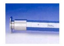
This hose is used for chemical transfer, pharmaceuticals, food processing and many other applications. Series RC is a smooth bore PTFE hose available in non-conductive or conductive PTFE. The outer jacket consists of two layers of Hypalon reinforced with fabric braid. A double steel wire helix supports the shape of the hose in full vacuum service applications.
