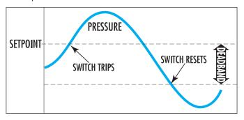
Chart shows hysteresis or "deadband" as a percentage of set pressure. Shows where electrical switch will de-actuate under falling pressure, after actuating at set pressure. This chart is a reasonable approximation of performance under laboratory conditions.
