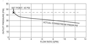
Droop is the difference between the pressure regulator set pressure and the actual downstream pressure at a higher flow. The chart above identifies the high flow capacities and the low pressure droop of Plast-O-Matic regulators which result in their greater sensitivity, finer adjustability and superior accuracy. The dashed line in the chart above represents the "theoretically perfect" pressure regulator; i.e., no droop regardless of flow rate.
