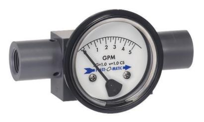
Plast-O-Matic flow gauges indicate liquid flow rates from low flows of 0-1 GPM to 0-10 GPM, even when used at high line pressures. Flow gauge sensors can be supplied with switches or relays to initiate alarms, activate other equipment, or shut the system down. Two switches are used when high and low limits are desired. Maximum line pressure rating is 200 PSI.
