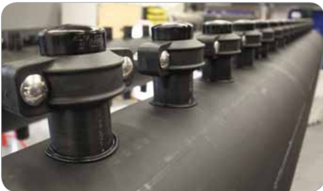
• 2" capped spigots on thermoplastic manifolds for membrane water treatment
