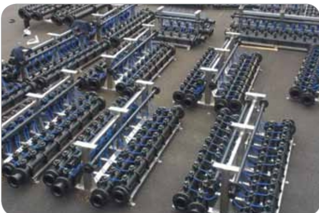
• Assembly of water purification manifolds Teblick Plastic Constructions & Installations Photo courtesy of Euro Mec
