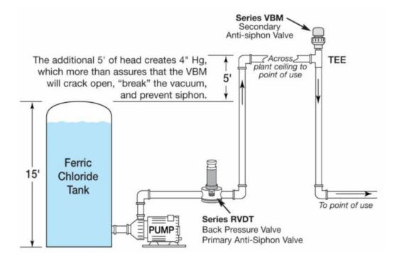
An engineering firm recently specified two seemingly unrelated Plast-O-Matic valves to provide redundant siphon prevention in a ferric chloride piping system.
