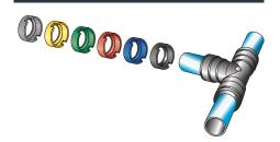
The slip-on Collet Cover shown in the illustration prevents accidental removal or tampering with tubing. Tubing can be inserted with the Collet Cover already attached to the fittings or the cover can slide into position afterwards. The cover is easily removed when required and comes in a variety of colors for color coding.
