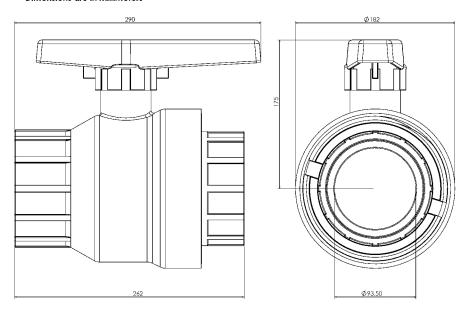
While other Ball Valves have a narrowed passage, the Netafim Ball Valve has a wide throat and clear pathway. This maximizes flow through when installed along a pipeline and increases flushing performance when installed on line ends.
