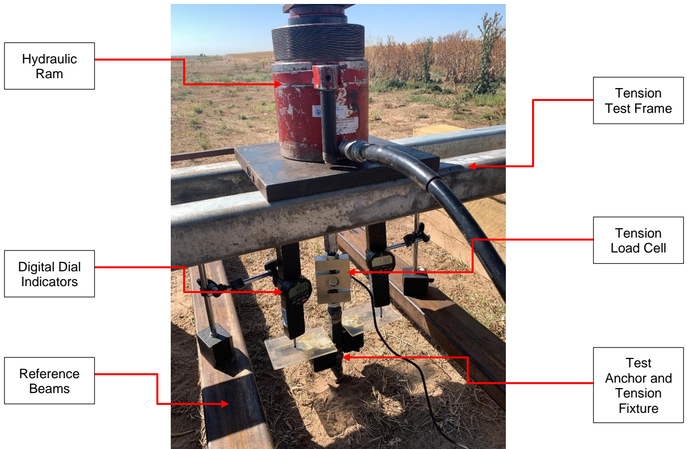
Figure 1. Tension Test Setup
