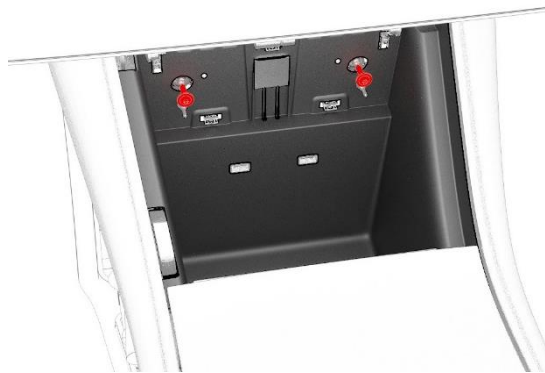
Figure 24. Center console front fasteners
