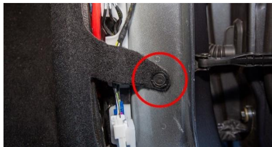
Figure 5. Detaching the RH passenger side carpet (RH carpet attachment shown for reference)
