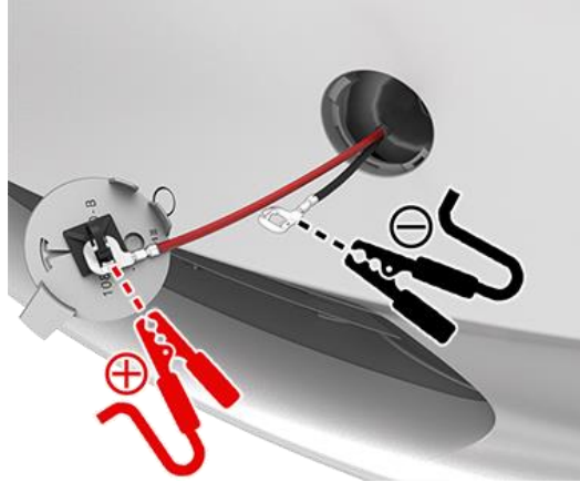
Figure 31. Connecting external 12V power to the Model 3 positive and negative terminals
