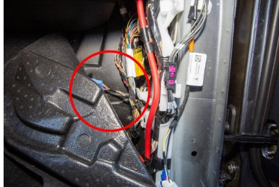
Figure 6. CAN bus connector location (RH location shown for reference)
