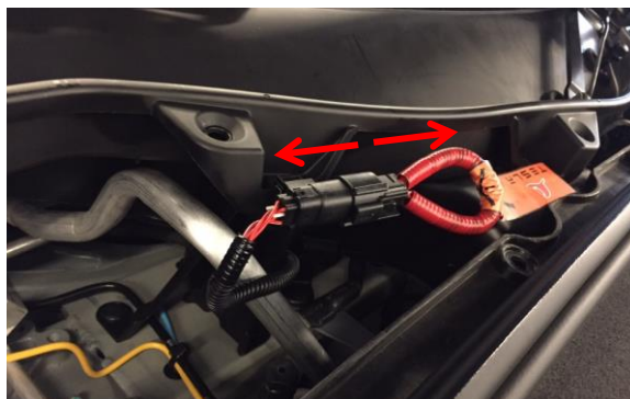
Figure 47. Disconnecting the first responder loop harness
