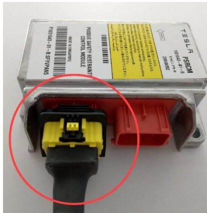
Figure 32. Connecting the EDR retrieval cable to the RCM (Vehicles built through February 25, 2019)
