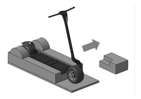
Remove the packaging from between the rear light vane and the rear tire.
