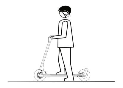
Once the scooter begins to coast, place both feet on the deck and gently press the throttle away from you to engage the motor. The eScooter motor will engage when the scooter exceeds 1.8 mph.
