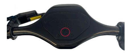
3.3.2 Switching Power Assist (PAS) levels When the display is on, single press the power button to switch the levels between ECO, D and S.
