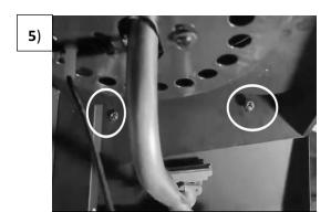
The final step is securing the screws circled above to the side burner
